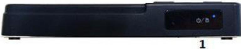
1. **LED indicators:** A blue light means the device is on. A blue blinking light means it is running low on memory.
