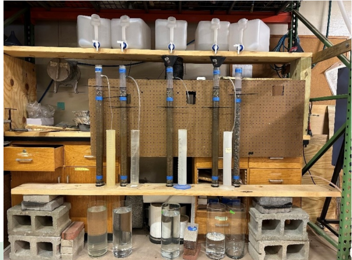
Figure 16: Picture of the constant head infiltration rate test being conducted at UNH in conjunction with the City of Dover Engineering Department.
