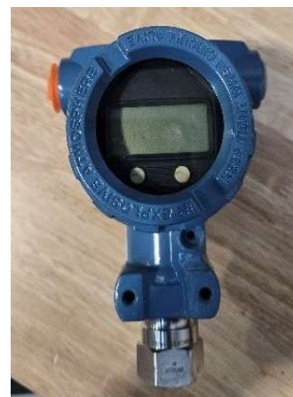
Figure 23: Level Transducer needing replacement.
