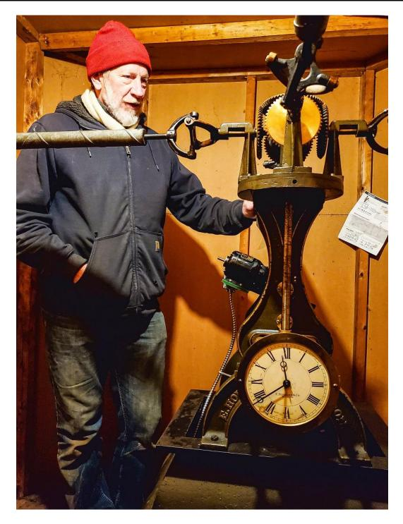
David Graf of Tower Clock Repair & Restoration explains how the clock mechanism works now with the repaired motor, and how it used to work when the clock was driven by weights.
