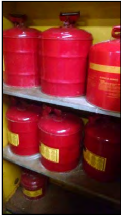
Flammables cabinet stored in the Maintenance garage.
