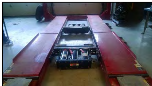
Hydraulic lift in auto shop.
