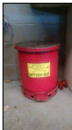
Oily solid waste receptacle in auto shop.
