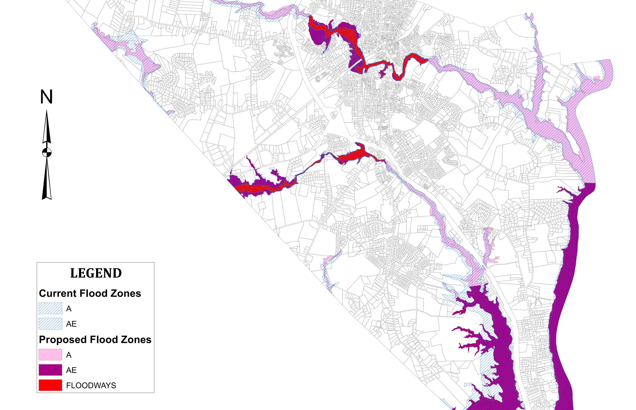
Note: Base Flood Elevation (BFE) is NOT established for A zones
