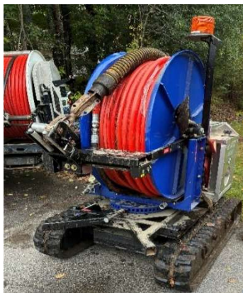
Figure 28: Sewer Easement Cleaning Machine.
