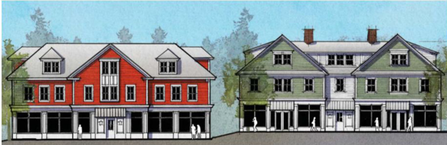
A complex of smaller scale buildings is preferable to a single large structure because the varied massing provides visual interest and human scale.
