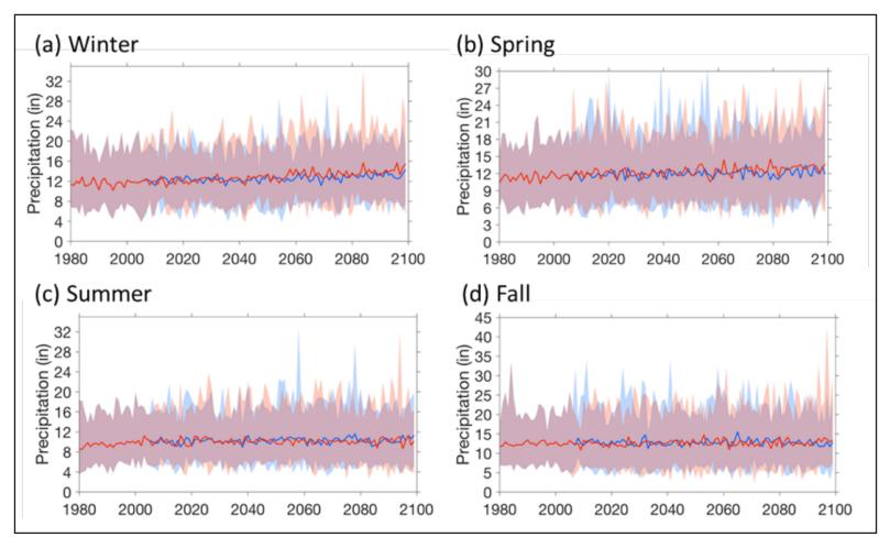
**Figure 7.5.** CMIP5 mean modeled historical (1980–2005) and projected future (2006–2099) total seasonal at Portsmouth, NH for (a) winter, (b) spring, (c) summer, and (d) fall for RCP4.5 (blue) and RCP8.5 (red) (from Burakowski et al., 2019.) Ensemble means are weighted following Sanderson et al. (2017).
